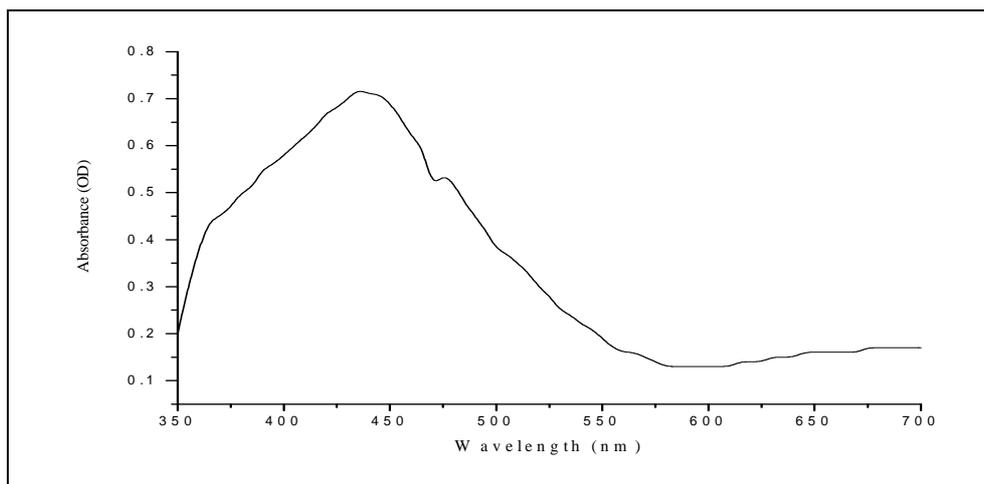
**Figure 2:** Absorbance spectrum of silver nanoparticles synthesized by *Lactobacillus sps* VRS2
