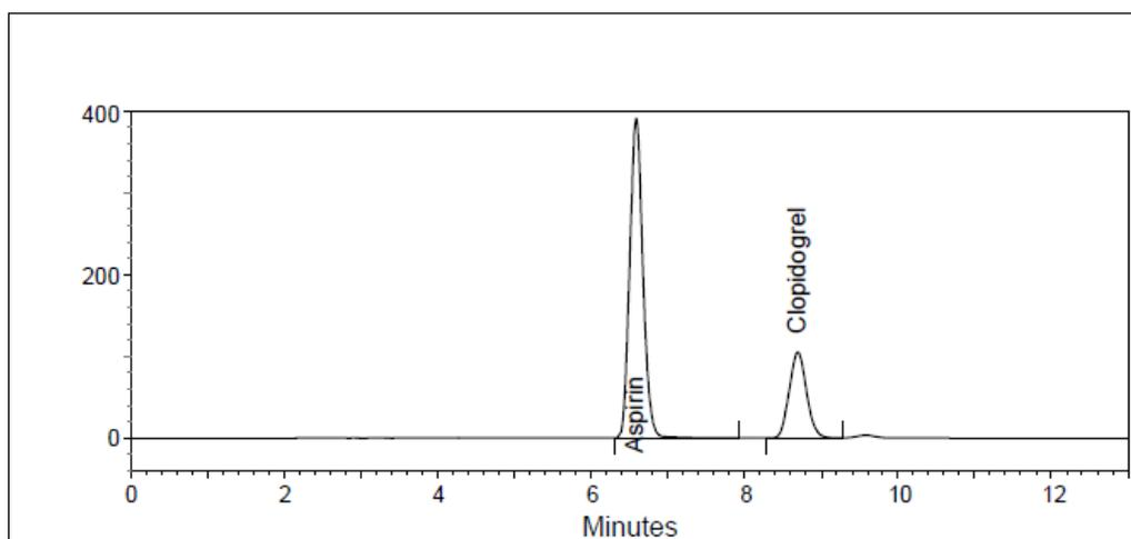
Figure 2. Chromatogram of test preparation (0.08mg/ml)
