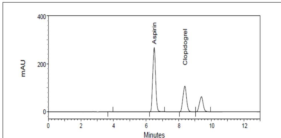
Figure 3. Chromatogram of acidic forced degradation study
